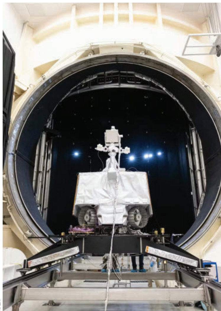
▲ NASA's VIPER (Volatiles Investigating Polar Exploration Rover) sits outside a testing chamber after completing its thermal vacuum testing in the fall of 2024.
